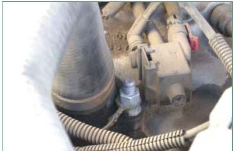
Figure 4: DRAC ground (G134) on thermostat housing bolt
