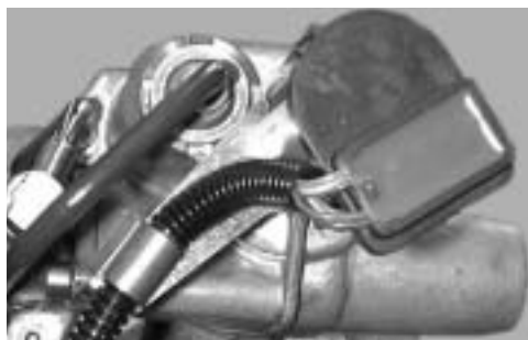
Position Sensor view from rear of Transmission
