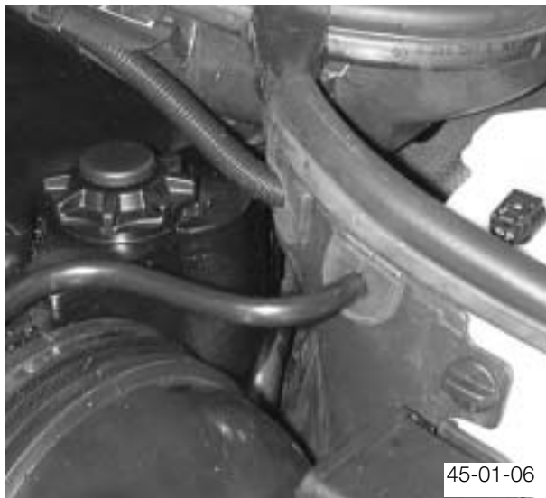
Hydraulic Fluid Expansion Tank Mounting
